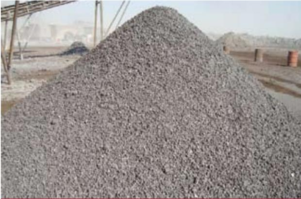
Crushed & Screened Slag for Downstream Use
