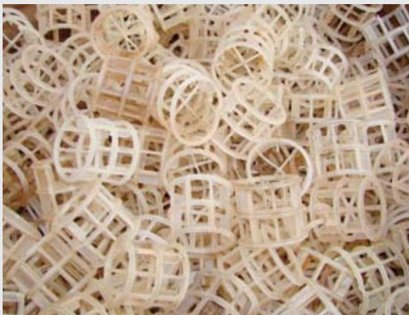
Vapour removal condenser packing was cleaned for the first time
