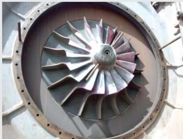
A new impeller was installed in the first stage process gas compressor
