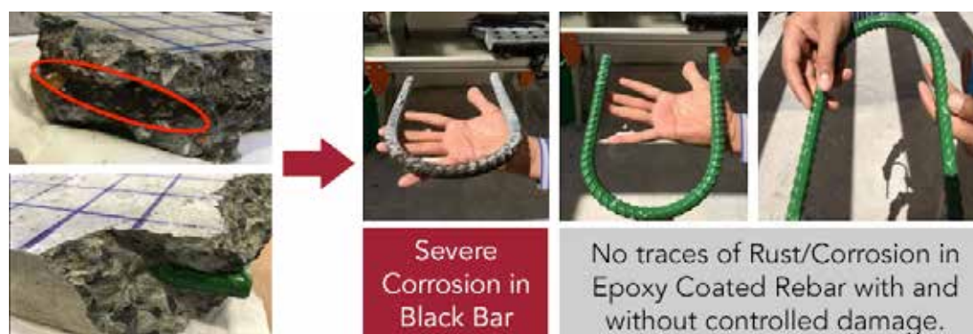
Condition of Rebar samples retrieved from concrete blocks after 2 years of exposure to continuous drying and wetting cycles in salt spray chamber (simulating actual Qatar Environment)
